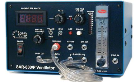
The Small Animal Ventilator, suitable for a mouse or guinea pig, operates as either a volume or pressure-cycled ventilator, meaning that it dispenses a designated volume of air with each breath or it ventilates until a designated lung pressure is reached. Pressure-cycled ventilation prevents hyper-inflation of small animal lungs.
