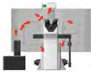
Fig. 1—Single air input and no venting causes random air flow in a traditional incubator.
