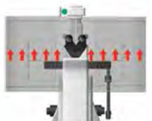
Fig. 3—A diffusion grid with air input and exhaust vents yields consistent air flow.
