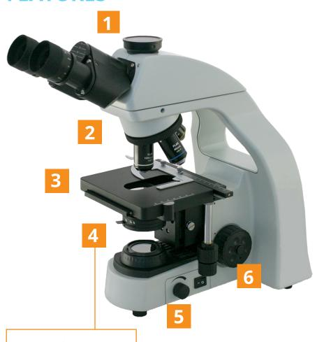
Ergonomically inclined trinocular head with eyetubes at 30° places user in the best working position, creating less tension and fatigue. Interpupillary distance is adjustable from 47~75mm. FPL-WF10x high eyepoint eyepieces, FN20. Eyepieces can hold a 20mm diameter reticle.
