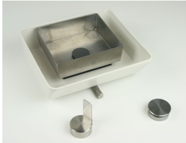
Inner and outer tissue bath (background) with standard tissue platen (front left) and adjustable tissue platen (front right)
