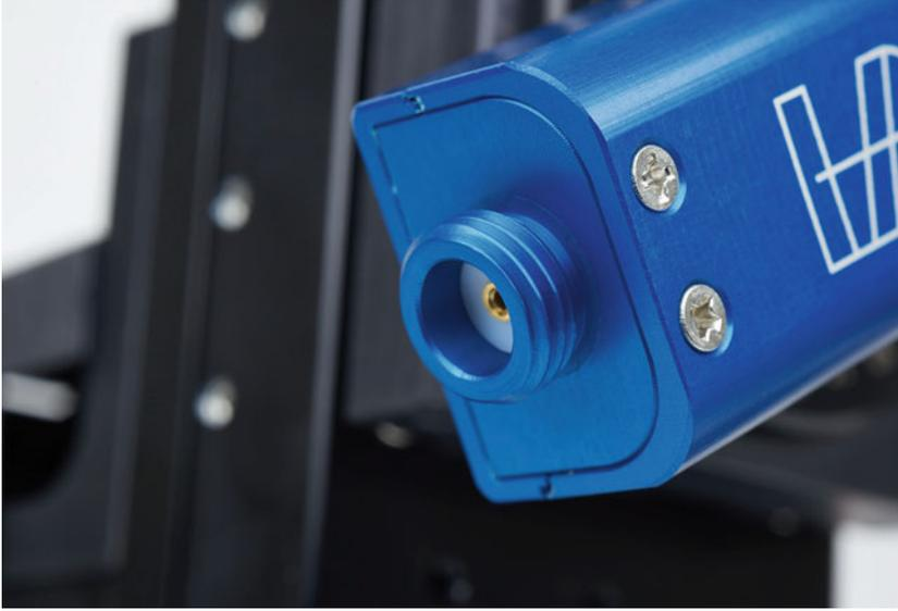
**Fig. 1** The pipette holder fitting on Sutter Instrument amplifiers is compatible with Axon Instruments' HL-U standard, which has been adopted by several other manufacturers. The threaded collar on Sutter headstages is executed in metal rather than the commonly used Teflon<sup>®</sup>. This provides both greater mechanical stability and better electrical shielding
