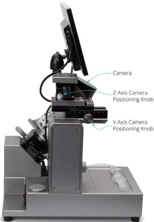
Fig. 6—Left side view of the Beveler showing the camera positioning knobs.
