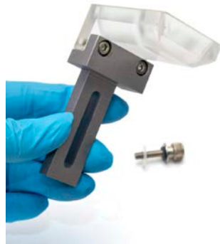
Fig. 39—Loosen the debris catcher adjustment screw while supporting the debris catcher. Fig. 40—The debris catcher was removed from the system.
