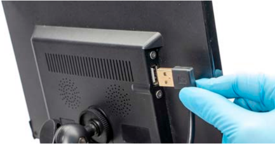
Fig. 24—Plug the USB type A connector from the camera into the port on the side of the monitor.
