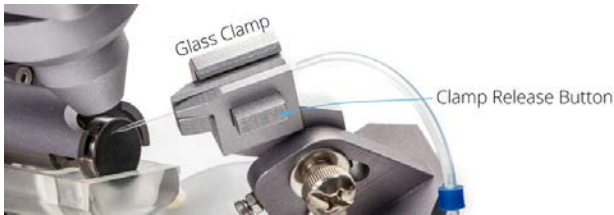
Fig. 11—Press and hold the clamp release button to install or remove a micropipette.
