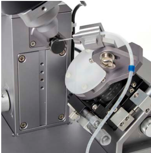
Fig. 41—The debris catcher was removed, revealing the four screw holes which give you options when reinstalling the debris catcher.
