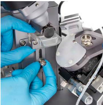
Fig. 39—Loosen the debris catcher adjustment screw while supporting the debris catcher. Fig. 40—The debris catcher was removed from the system.
