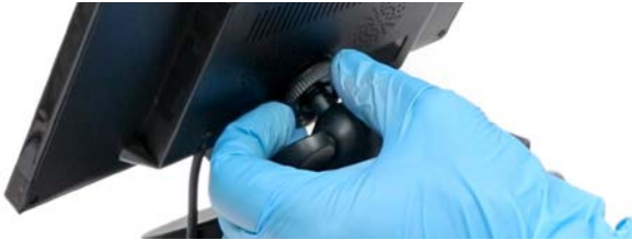
Fig. 22—Rotate the tightening wheel clockwise to secure it.
