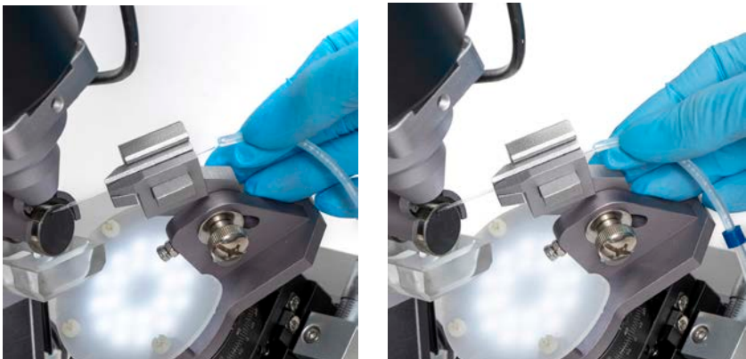
Fig. 37—Slide the tubing on the blunt end of the pipette.
