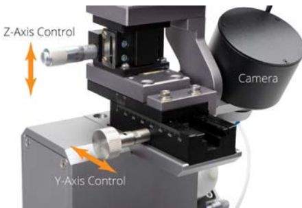
Fig. 7—These controls are used to position the camera lens.
