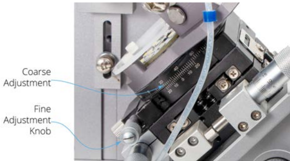
Fig. 12—The black rotary platform may be tuned to precisely set the beveling angle.
