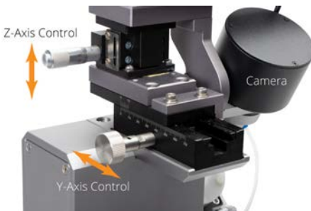
Fig. 33—These controls are used to position the camera lens.
