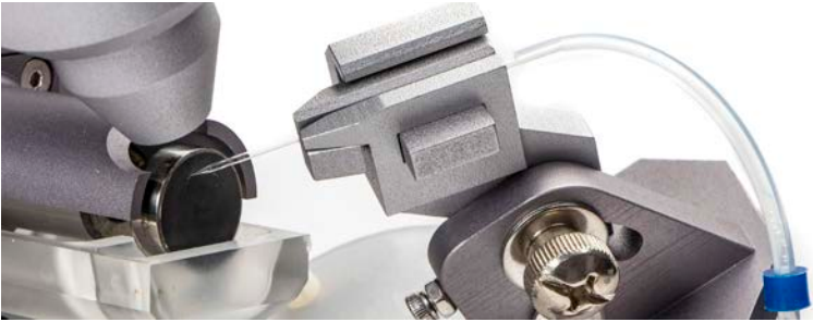
Fig. 38—The tubing fits over the blunt end of the micropipette so you can push water through the tip and into the acrylic cup below the diamond wheel.
