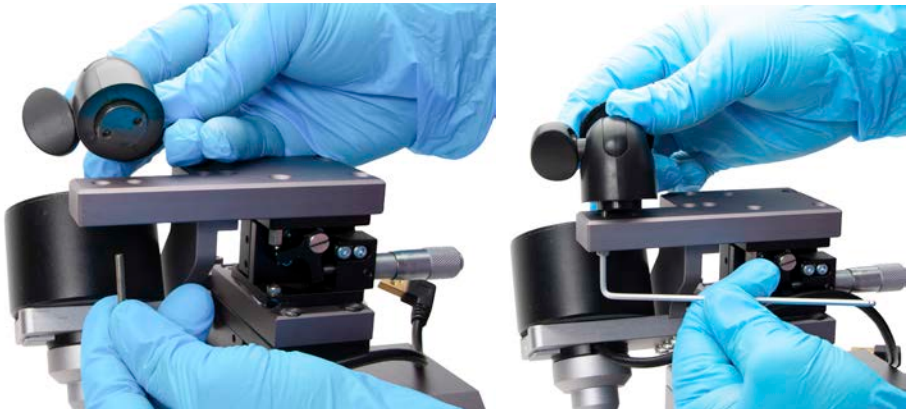
Fig. 19—Insert the first mounting screw through the bottom of the mounting arm and into the corresponding hole in the mounting head.
