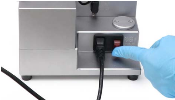
Fig. 28—Turn on the power switch on the back of the Beveler.
