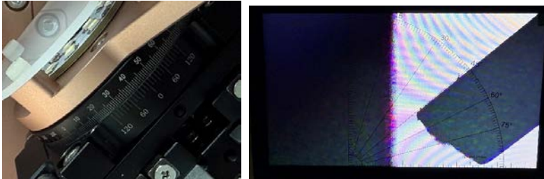
Fig. 32—Here you see 45° on rotary platform and 45° on the monitor's angular scale.
