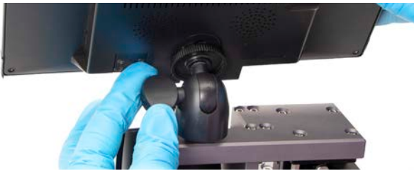
Fig. 23—Rotate the knob counter clockwise to loosen it. Then position the angle of the monitor as desired. Rotate the knob clockwise to secure the monitor angle.
