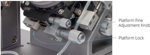
Fig. 10—Adjust the fine tuning on the rotational platform and twist the platform lock to secure the position.
