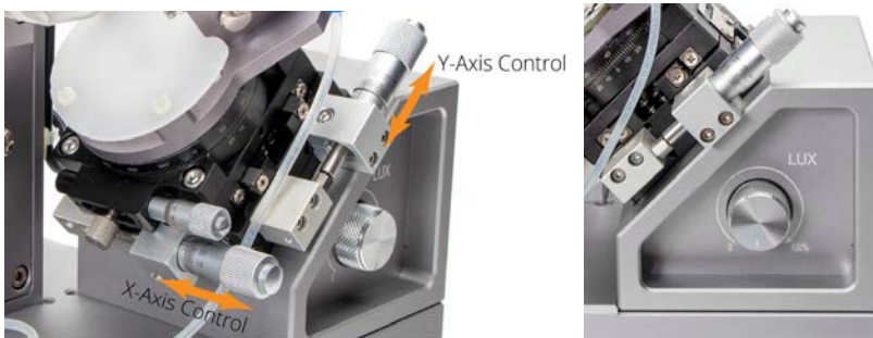
Fig. 13—(Left) The X and Y Axis Adjustment Knobs control the position of the micropipette.
