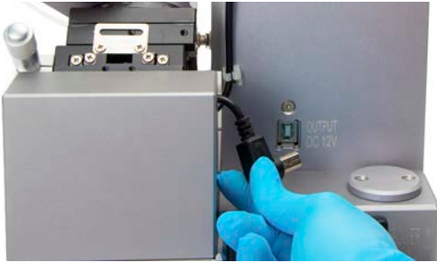
Fig. 25—Plug in the power cable from the monitor into the USB (type B) port on the back of the Beveler.
