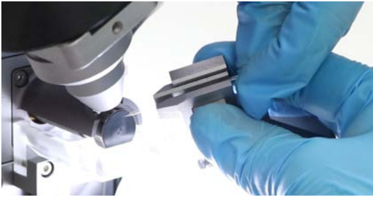
Fig. 29—Pinch and hold the release button and install the glass.
