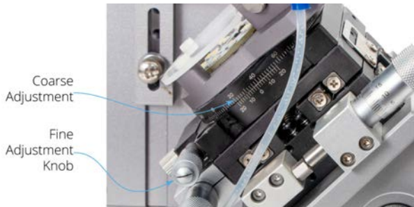
Fig. 30—The black rotary platform may be tuned to precisely set the beveling angle.
