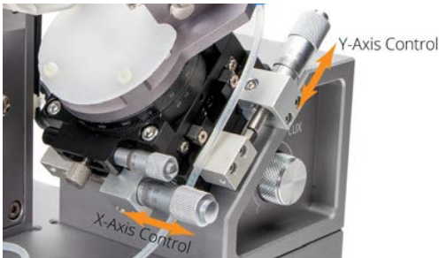
Fig. 34—The X and Y-Axis Adjustment Knobs control the position of the micropipette.
