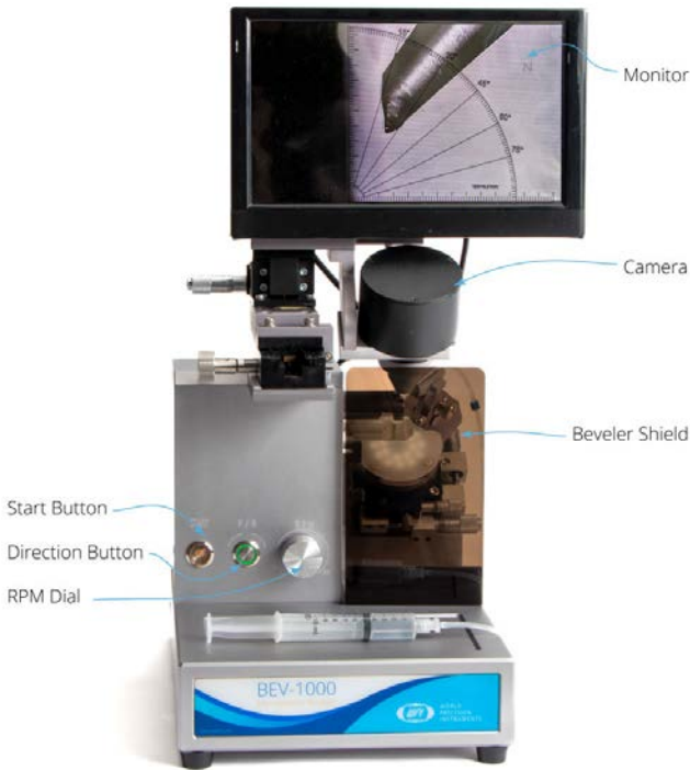
Fig. 2— The front view of the Beveler.
