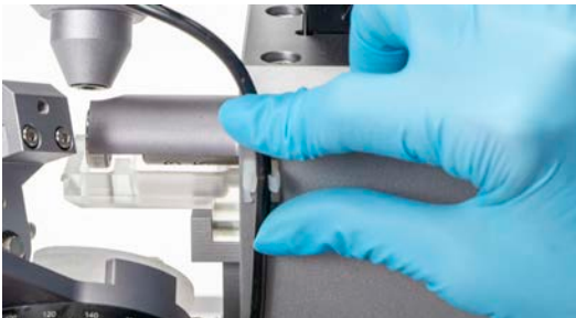
Fig. 26—Snap the cable into the two cable holders on the back of the Beveler to keep them out of the way during operations.
