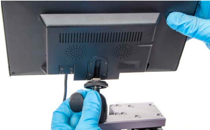
Fig. 21—Position the monitor so that the metal attachment insert aligns with the receptacle on the back of the monitor.
