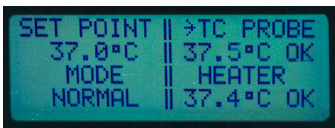
Fig. 7—The home page display shows the set point, mode, control temperature and plate temperature.
