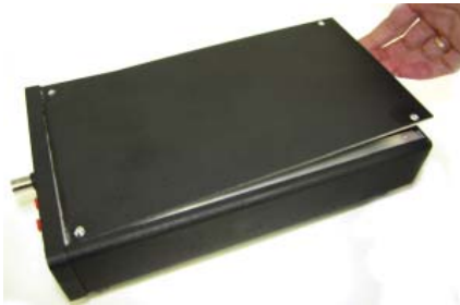
Fig. 7—If you tip the box upside down, the back end of the lid opens and you can slide it off the box.
