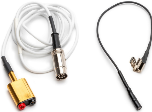
Fig. 5—(Left) CardioPhys™ ECG probe with head stage
