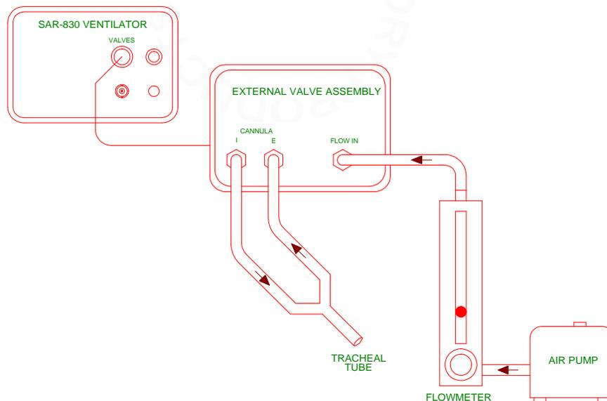
*Figure 2: Expanding the SAR-830 with an EXTERNAL VALVE ASSEMBLY*
