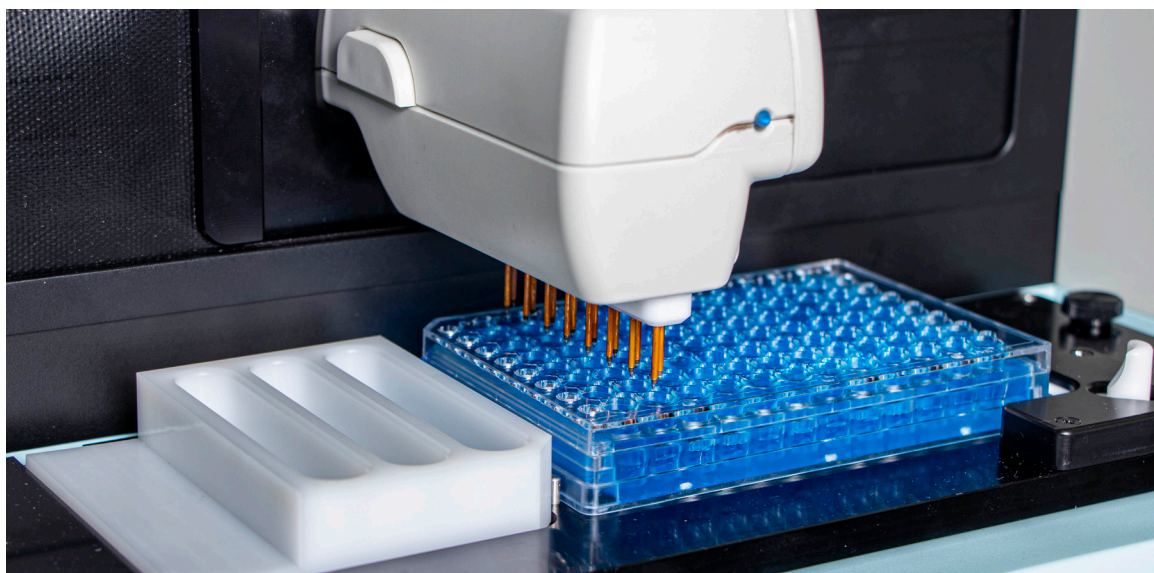
The electrode array positions eight pairs of electrodes precisely in the wells and measures a column at a time, each well sequentially. As measurements are made, they appear on the iPad screen in real time.
