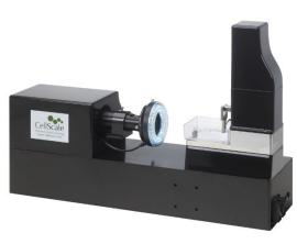
MicroTester G2 – High-precision Micro-scale Mechanical Testing
