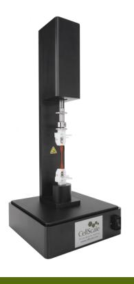
UniVert – Uniaxial Tension, Compression and Bending Testing
