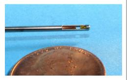
This tiny shaft contains 14 fused silica fibers, all polished to a perfect tip. Light travels through seven fibers through the sample. It is reflected off a mirror in the tip and returns to the spectrometer through the sample and the other seven fibers.
