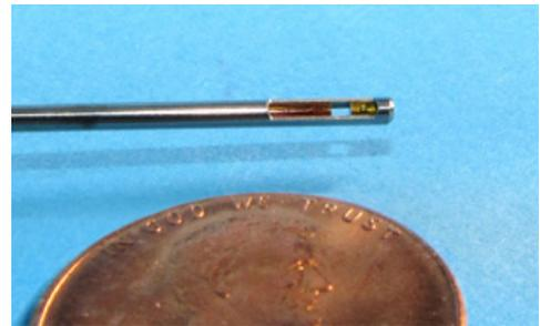
*This tiny shaft contains 14 fused silica fibers, all polished to a perfect tip. Light travels through seven fibers through the sample. It is reflected off a mirror in the tip and returns to the spectrometer through the sample and the other seven fibers.*
