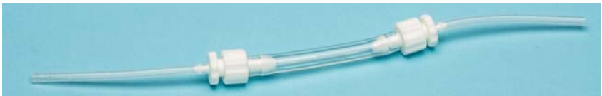
Fig. 14— The overflow adapter has two luer fittings used to connect to a syringe.
