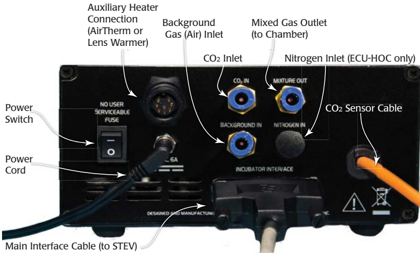
Fig. 7—The ECU-HCP back panel has the ports and connectors to connect the STEV chamber with the electronic controls. The ECU-H5 has no Gas Inlet port or CO 2 Sensor Cable. Because the ECU-HC has an internal sensor, it will not have a CO 2 Sensor Cable. The ECU-HOC has an additional port for nitrogen inlet.
