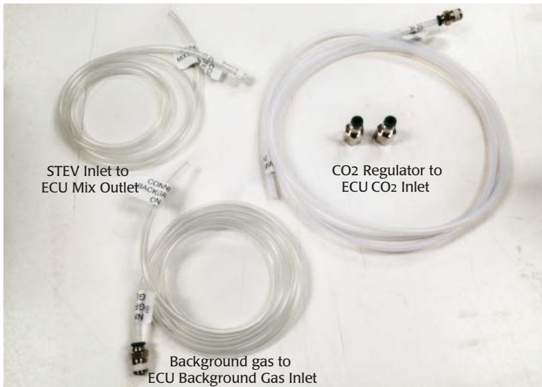
Fig. 8—The tubing kit contains all the tubing to connect the gas tanks, the ECU and the STEV. This kit will vary somewhat depending on which ECU you ordered.
