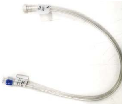
Fig. 16—The white end of the reservoir filling tube attaches to the STEV water intake tubing, and the blue end attaches to a syringe.
