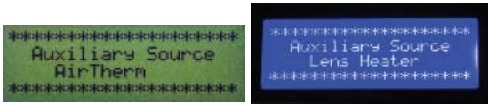
Fig. 52—Choose AirTherm or Lens Heater by pressing the Up or Down button.
