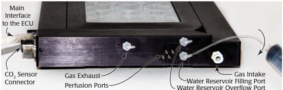
Fig. 18—The ECU-HCP (shown) has the connector for the external CO 2 sensor.
