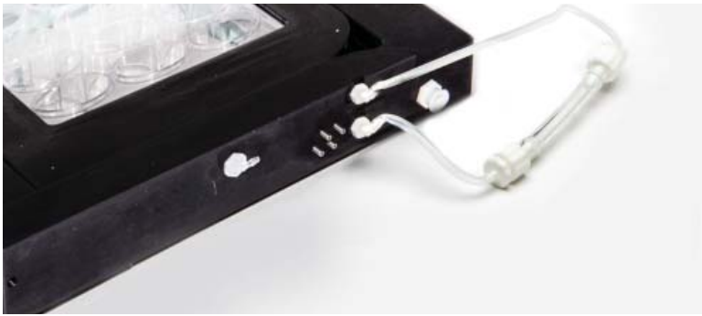
Fig. 15—The overfill adapter is connected to the STEV filling and overflow ports.
