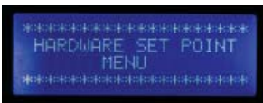
Fig. 46—Press the Up and Down buttons together to enter the Hardware Setpoint menu.
