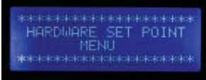
Fig. 51—Press the Up and Down buttons together to enter the Hardware Setpoint menu.
