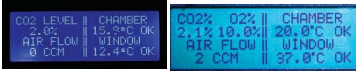
Fig. 24—(Left) The default display of the ECU controller continuously updates to show four measured parameters. The ECU-H5 displays “None” for the CO 2 value, because a pre-mixed gas of known concentration is used, and CO 2 is not monitored.
