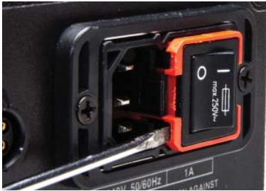
Fig. 57—(Left) Insert the screw driver under the fuse housing lip and pry the housing open.
