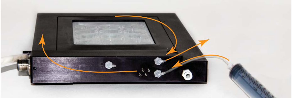
Fig. 4—Use a large syringe filled with distilled water to fill the water reservoir. When it is full, water will come out the overflow port.
