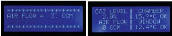
Fig. 30—(Left) Press the Air button to display only the current air flow to the chamber.
