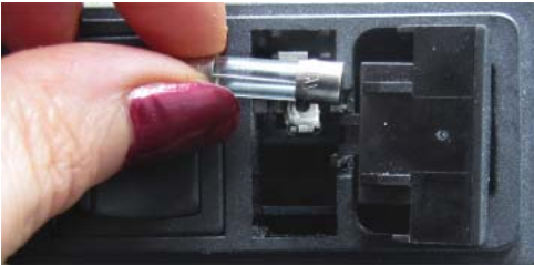
Fig. 62—Open the fuse housing and rotate it right to remove the fuse.
