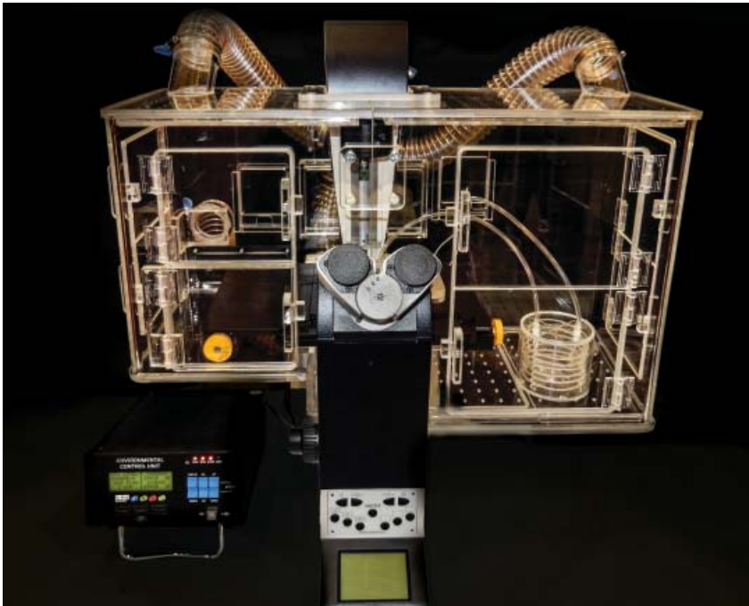
Fig. 2—A complete environmental control system includes the ECU (Environmental Control Unit), a microscope with chamber and a STEV stagetop environment.
