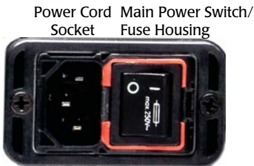
Fig. 56—Unplug the power cord to access the fuse housing release.
