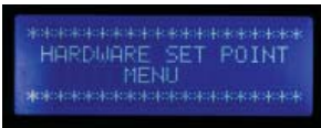
Fig. 49—Press the Up and Down buttons together to enter the Hardware Setpoint menu.
