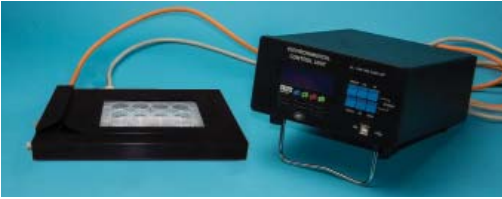
Fig. 1—The Stagetop Environment (STEV) and ECU (Environmental Control Unit) comprise the basic incubator system for growing cells under controlled conditions.
