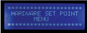
Fig. 44—Press the Up and Down buttons together to enter the Hardware Setpoint menu.
