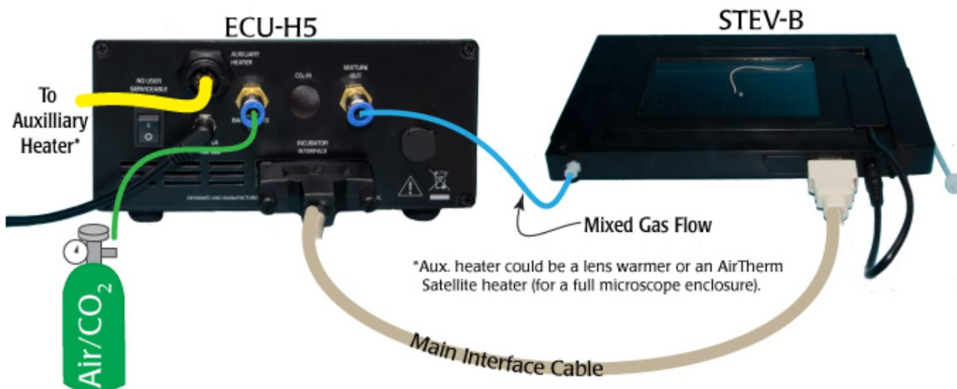
Fig. 4- The ECU-H5 connections
