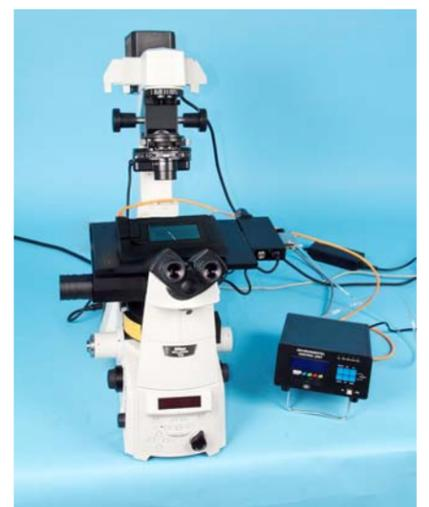
A complete stagetop environmental control system includes the ECU (heat/CO<sub>2</sub> controller), and the STEV stagetop environment.
