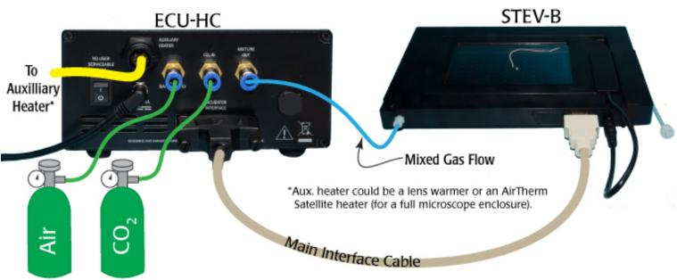
Fig. 3- The ECU-HC connections.
