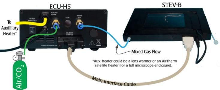
Fig. 4- The ECU-H5 connections
