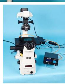
A complete stagetop environmental control system includes the ECU (heat/CO<sub>2</sub> controller), and the STEV stagetop environment.
