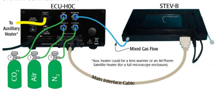
Fig. 1- The ECU-HOC connections
