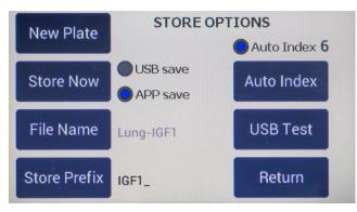
• The EVOM™ Manual can temporarily hold data for up to three plate files internally in a queue before the data can be exported into the USB flash drive or to the EVOM™ Companion App. Thus, data for up to three data files can be uploaded to the desired storage location.
