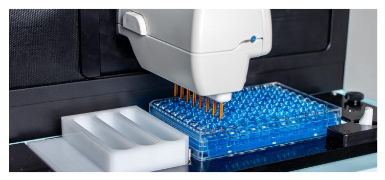
The electrode array positions eight pairs of electrodes precisely in the wells and measures a column at a time, each well sequentially. As measurements are made, they appear on the iPad screen in real time.
