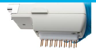
The EVA-EL-03-01 electrode array has 8 pair of (1.25mm  $\Phi$ ) electrodes, which are specially designed to fit precisely in 96-well plates, ensuring consistent placement. It performs resistance measurements directly in the plate, common or divided, reducing the possibility of contamination and mechanical damage to your cultured cells.
