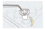
To conduct the media exchange, inserts must be lifted one at a time, using tweezers or other tools, which is labor-intensive process.
