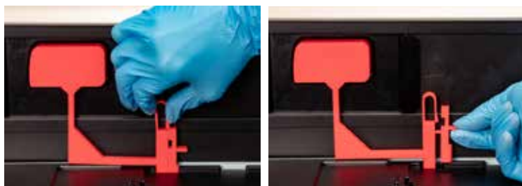
Fig. 15—(Left) Pinch the latch at the top of the lock.
