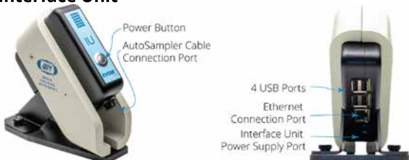
Fig. 8—(Left) Side view of the interface unit, showing the front.
