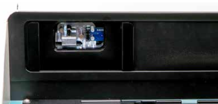
Fig. 22—The electrode array connection port is on the back wall of the autosampler.
