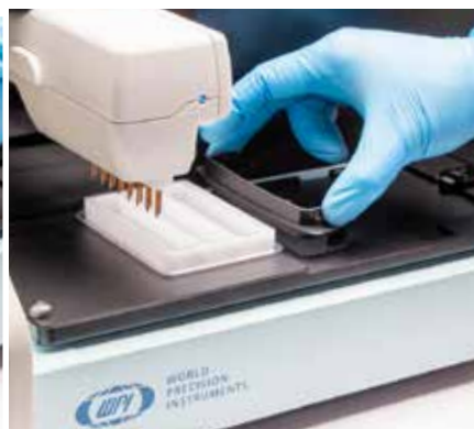
Fig. 36—Lightly press the plate positioner and plug the plate positioner in place.
