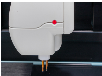
Fig. 22—The electrode array LED is illuminated red.
