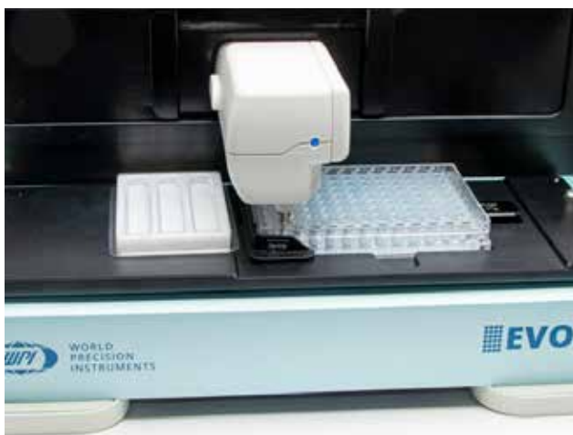
Fig. 60—The electrodes are properly placed in the well plate.
