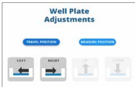
Fig. 56—In the Well Plate Adjustment Area , press the Travel Position button.
