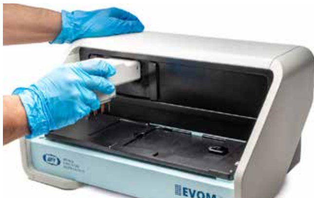
Fig. 23—Hold the top of the autosampler with one hand, line up the electrode array with the connection port and press the electrode array into the connection port until it clicks.
