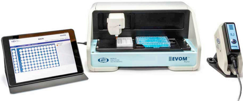
Fig. 1—The EVOM™ Auto with 96 high throughput screening (HTS) electrode array simplifies transepithelial electrical resistance (TEER) measurement in 96-well HTS plates from MatTek, Corning, and Millipore multiwell plates. The system is also available for 24-well plates.
