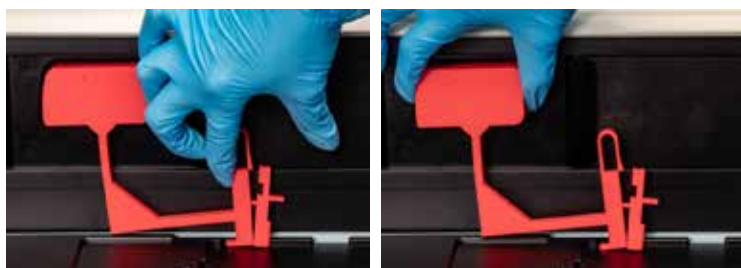
Fig. 17—(Left) Push the locking mechanism till the clasp releases from the slot in the base.
