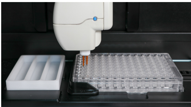
Fig. 55—Make sure the electrodes align with the holes in the well plate.
