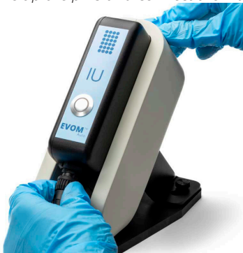
Fig. 8—Line up the pins and connect the interface cable to the interface unit.
