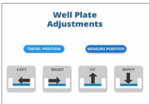
Fig. 58—In the Well Plate Adjustment Area, press the Travel Position button. After pressing the TRAVEL POSITION button only the left and right arrows are operational. The up and down arrows are greyed out
