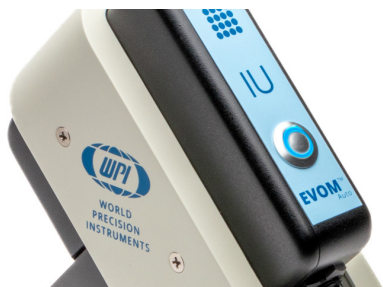
Fig. 23—The blue ring illuminates around the power button when the unit is powered on.
