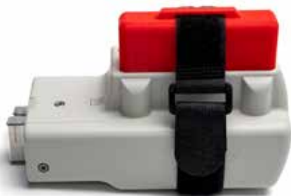
Fig. 20— The electrode array is packaged with a protective sleeve secured with a heavy Velcro strap.
