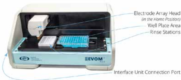
Fig. 3—The autosampler takes the TEER measurements of the HTS well plate.
