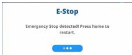
Fig. 52—After an emergency stop is detected, your only option is to send electrode array to the home position. Make sure the well plate is sitting flat onto the base and the correct plate is being used.
