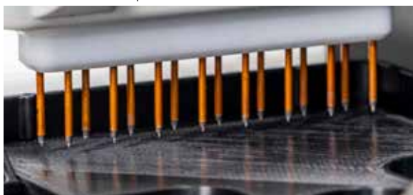
Fig. 57—The electrode tips should be positioned above the plate, but should not touch it.
