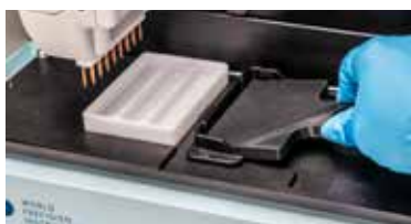
Fig. 43—Install the depth adjustment fixture where a well plate would go.
