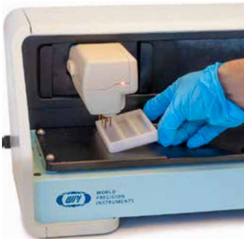
Fig. 32—(Left) Slide the rinse station into the pocket.
