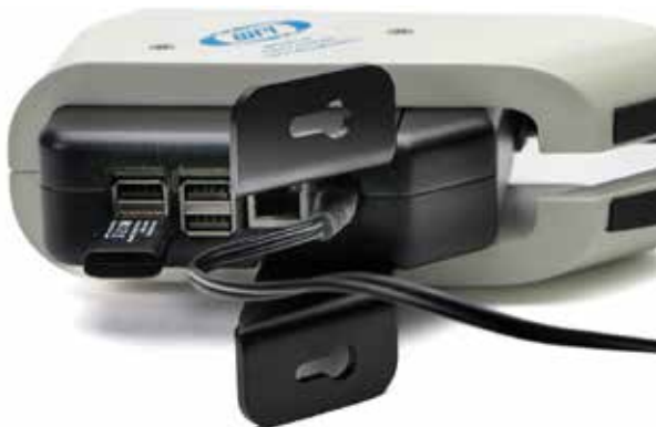
Fig. 12—Connect the power cable to the interface unit.
