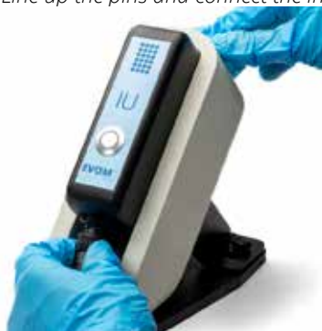
Fig. 11—Line up the pins and connect the interface cable to the interface unit.
