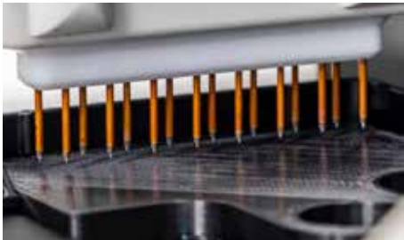
Fig. 44—The tips of the electrodes should stop just above the alignment tool without touching.
