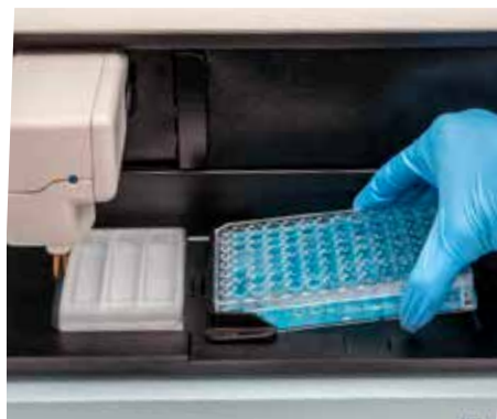
Fig. 37—(Left) Let the left side of the well plate (A1) rest on the base.
