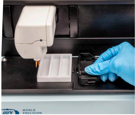
Fig. 32—Lightly press the plate positioner and plug the plate positioner in place.
