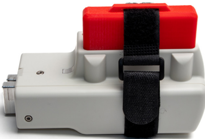
Fig. 17— The electrode array is packaged with a protective sleeve secured with a heavy Velcro strap.
