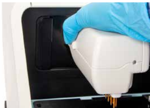
Fig. 24—Depress the button on the left side of the electrode array until you hear a click. Then, pull the array out to remove the electrode array. No light on the electrode array indicates the unit is off, and a red light on the electrode array indicates you are in offline mode. In either case, it is safe to remove the electrode array.
