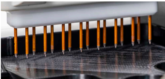
Fig. 53—The electrode tips should be positioned above the plate, but should not touch it.
