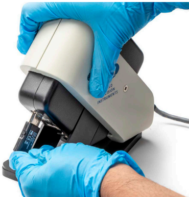
Fig. 10—The Wi-Fi adapter is installed in one of the four USB ports on the back of the interface unit.
