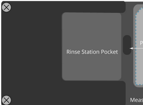
Fig. 30—The rinse station is positioned in the Rinse Station Pocket.
