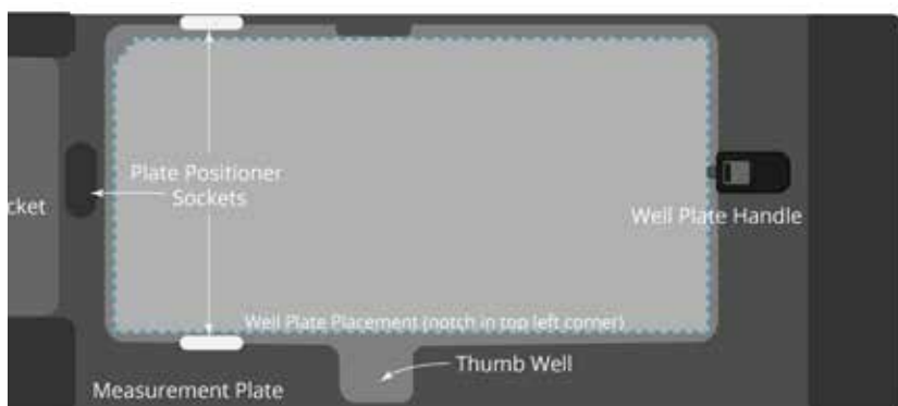
Fig. 39—Use the plate positioner to align the well plate.
