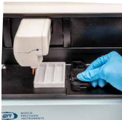
Fig. 47—Plug the plate positioner into the slot. The plate positioner helps to keep the well plate properly aligned on the base.
