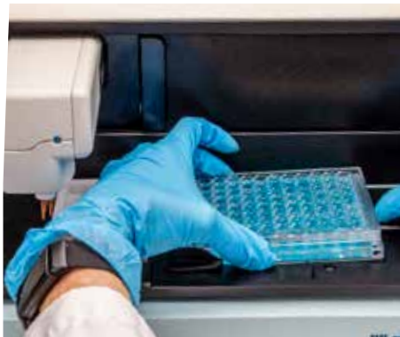
Fig. 37—(Left) Let the left side of the well plate (A1) rest on the base.
