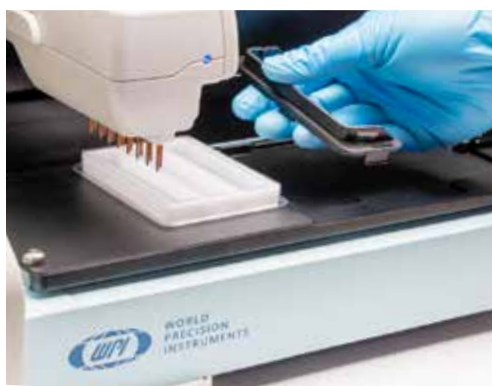
Fig. 35—Identify the slot to plug in the plate positioner
