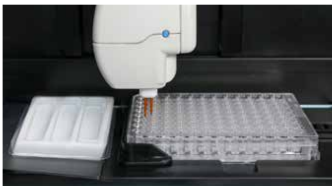
Fig. 59—Make sure the electrodes align with the holes in the well plate.
