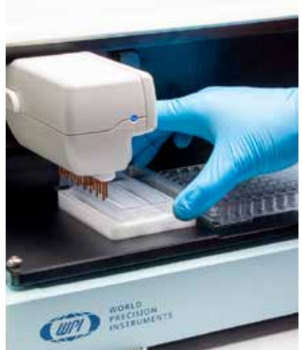
Fig. 33—(Right) Insert a sterile disposable rinse station insert in the base rinse station.
