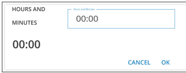
Fig. 58—(Left) If you select the pencil icon, you may use the keyboard to enter a four-digit number in the form of HHMM to set the period.
