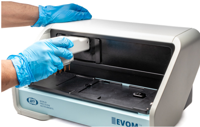
Fig. 19—Hold the top of the autosampler with one hand, line up the electrode array with the connection port and press the electrode array into the connection port until it clicks.
