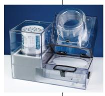
The BioVac Chamber option, a self contained, laminar-flow system, virtually eliminates the release of isoflurane into the room.
