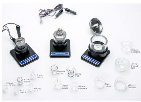
height of the top electrode can be adjusted to fit cell culture cups of different manufacture.
