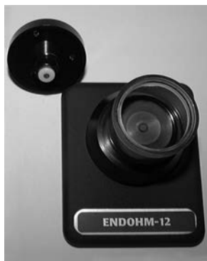
Fig. 4—(Left) ENDOHM-12G shown that has not been chlorided enough
