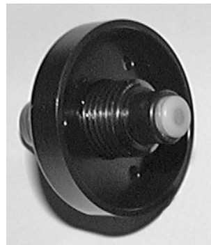
Fig. 6—(Left) A clean EndOhm surface with no spots or irregularities
