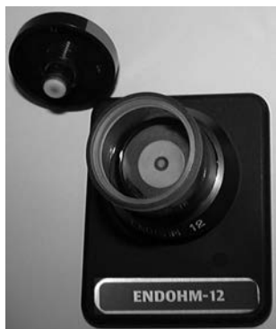
Fig. 4—(Left) ENDOHM-12G shown that has not been chlorided enough
