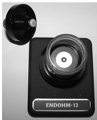
Fig. 6—(Left) A clean EndOhm surface with no spots or irregularities
