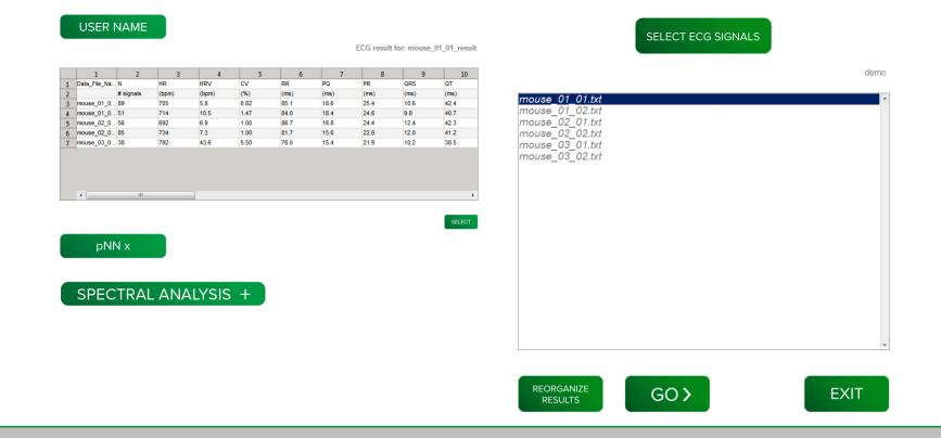
The Main Graphical User Interface of the companion ECG analysis software asks the user to specify a directory and ECG files to be analyzed. The user can choose the option to perform heart rate variability (HRV) analysis in the frequency domain.
