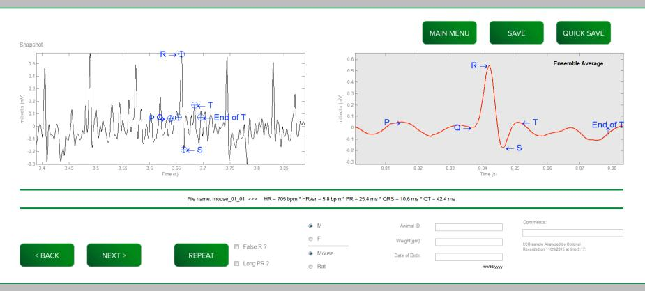
A snapshot of the signal is provided, showing the PQRST morphology for one of the complexes. Here the user has the option of entering animal demographics. Imagine after scores of recordings an ample database for normative control values, to reduce the numbers of animals and experiments needed for future studies. *These data are from conscious mice without surgery or implants.*
