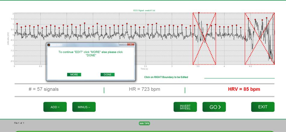
The raw ECG signal is presented, including any baseline drift and artifacts. Feedback is provided to the user regarding the quality of the data and number of complexes desired for analysis. The user is equipped with tools to extract from the signal noise associated with animal movement.
