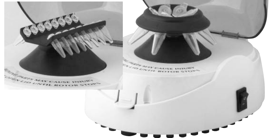
Fig. 1 – gSpin. Inset shows alternate rotor style for PCR strips.
