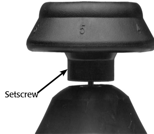
Fig. 4 – PCR rotor with Allen wrench in setscrew
