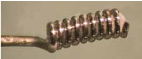
Fig. 2 – Tip of the sensor showing the coil holding the enzyme saturated cotton plug. The diameter of the coiled tip is about 600 \mu m.
