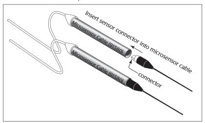
Fig. 1–ISO-HPO-100 microsensor with cable
