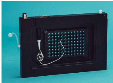
The base unit above has the lid removed, showing the placement of the temperature sensor in one of the wells of a 96-well plate.
