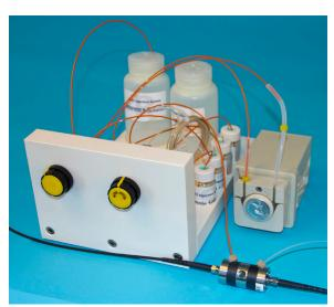
The sample measurement procedure can be improved using the optional LWCC Injection system (WPI # 89372) as discrete, reproducible sample volumes can be introduced to the LWCC-M with a seamless transition from the baseline solution to sample at a continuous flow rate. The LWCC Injection System, together with a pump and liquid waveguide capillary cell (LWCC-M), provides an efficient, continual flow for injecting a sample through the **LWCC-M**.
