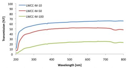
Fig. 4—This graph show the percentage of light transmission at various wavelengths. The higher the light transmission percentage, the greater the resolution.
