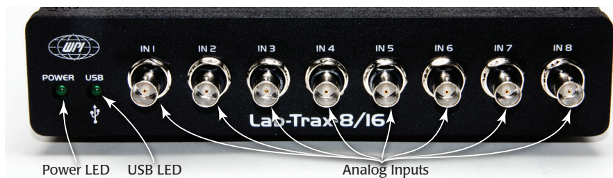
Fig. 14—The front of the LabTrax 8/16 has eight analog inputs.
