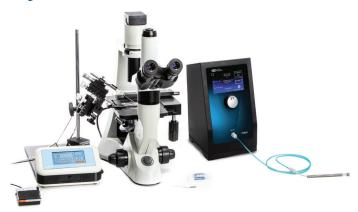
A typical microinjection setup with the MICRO-ePORE™, an INV-101 Inverted Microscope and a PV820 Pneumatic PicoPump.
