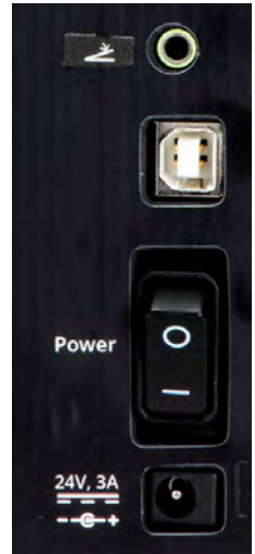
Fig. 3—The Interface Cable Connector is labeled “Front Panel.” Do NOT plug it into the foot switch port on the rear panel.
