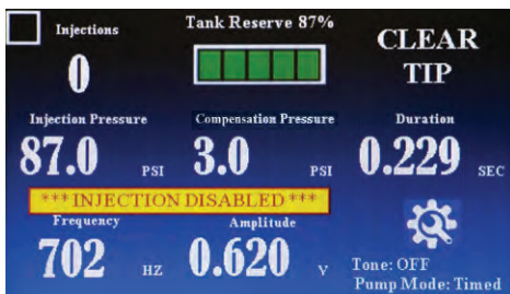
Fig. 10—The warning indicates that the injection port is disabled by default on startup.
