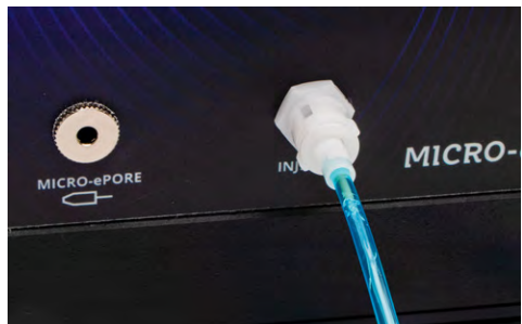
Fig. 12—(Left) Align the connector with the Injection Port, slide the connector in position and rotate the connector a little clockwise to lock it into place.
