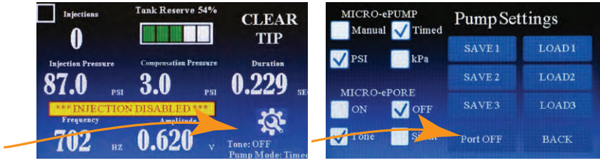
Fig. 19—(Left) Touch the setting area in the bottom right corner to access the Settings menu. Fig. 20—(Right) Touch the Port OFF button to enable the injection port.
