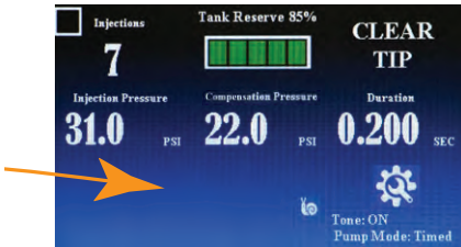
Fig. 23—The MICRO-ePORE™ is disabled in this configuration. No parameters show in the bottom half of the screen.
