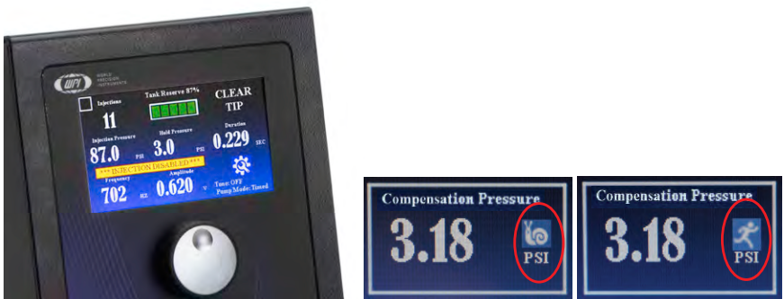
Fig. 21—(Left) Touch the parameter to adjust and rotate the knob to modify the parameter. Fig. 22—(Right) Press the knob to toggle between gross and fine tuning adjustments.
