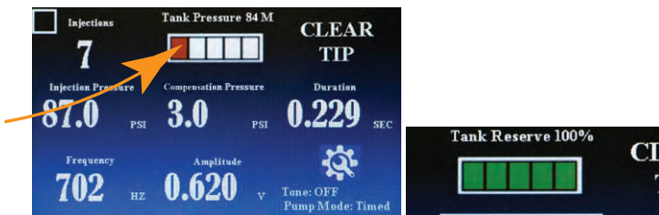
Fig. 27—(Left) Touch the gauge to start refilling the reservoir.
