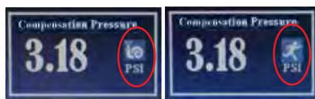
To change the dial adjustment speed, press the knob on the front of the MICRO-ePUMP. The snail changes the display in 0.01 increments, and the running man changes it in increments of 0.1.
