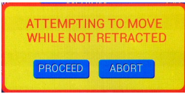
Fig. 33–If the present position is below the retracted position, you will get this warning message when you attempt to move the axes in the AP-ML plane.
