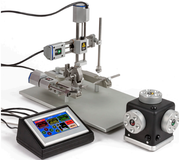
Fig. 1—The MTM-3 motorized stereotaxic frame comes with the touch screen controller (left). An hand controller (right) is also included.
