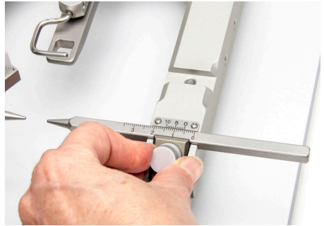
Fig. 15—(Left) Mount the ear bars so the numbers are right side up.
