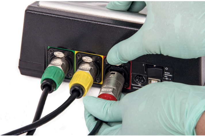
Fig. 20-Depress the button, line up the arrow at the top and slide the cable for the axis control into its color-coded port.
