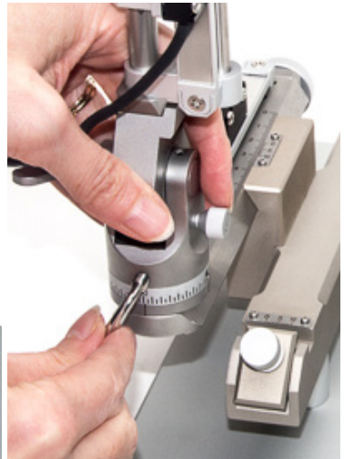
Fig. 9-(Left) Position the turret over the post and slide it into place.
