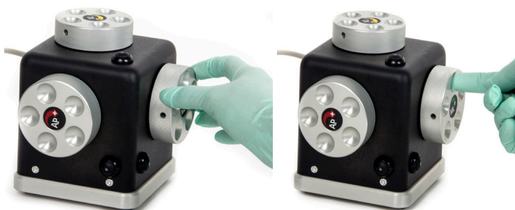
Fig. 36–(Left) Rotate the dial for the appropriate axis to move that axis.
