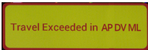
Fig. 47–A warning displays when you command the MTM-3 to move to coordinates outside the range of travel of any axis.
