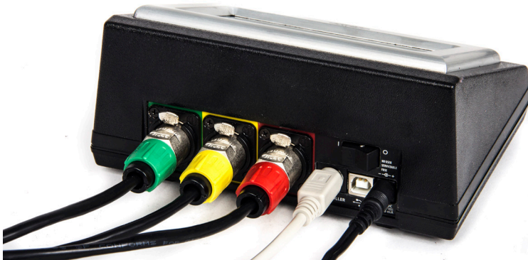
Fig. 21-This control box is connected to the three axes, the hand controller and the power supply.
