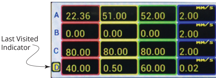
Fig. 46–The highlighted letter indicates the programmed coordinates that were used last.
