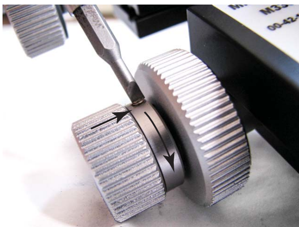
Fig. 10—The flat blade of the screwdriver should be positioned perpendicular to the adjustment ring to make the ring easier to rotate.
