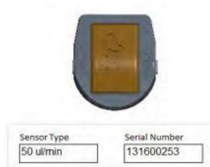
Displays information regarding the flow sensor: the flow rate range and the serial number.
