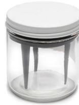
**MicroFil** is a flexible and reusable glass needle as small as 36 gauge for backfilling micropipettes.
