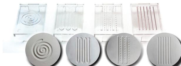
**Z-MOLDS** Microinjection and Transplantation Molds (4 per kit) are designed for zebrafish research. The molds are turned up-side down and placed in liquid agarose gel and are easily removed once it has solidified. Pipette the embryos into the grooves. The embryos self-align.
