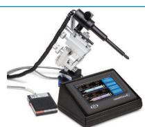
Microprocessor-controlled Nanoliter Injector **NL2010MC2T** with SMARTouch controller uses positive displacement injection, eliminating the need for pipette calibration. System uses glass micropipettes.
