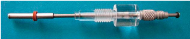
Fig. 6 —The mounting tube with the gasket slides over the membrane sleeve.
