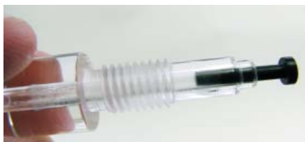
Fig. 2—Installing the Side Fitting Plug.
