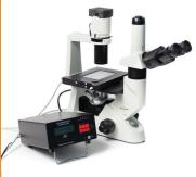
A microscope stagetop incubator is perfect for adding Live Cell Imaging to an existing microscope. The **STEV2** incubator with the stagetop environmental control system is a compact environmental case to house your culture wells and control for heat, humidity, CO<sub>2</sub> and O<sub>2</sub>.
