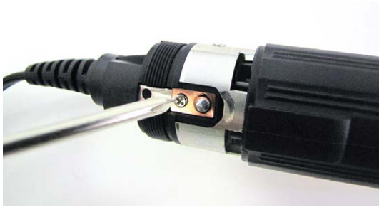
Fig. 10—Use a screwdriver to remove carbon brushes
