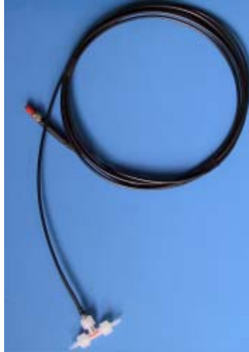
Flow through cell design connected to a 2 mm POF
