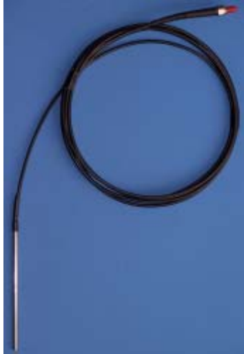
2 mm POF with coated sensor foil
