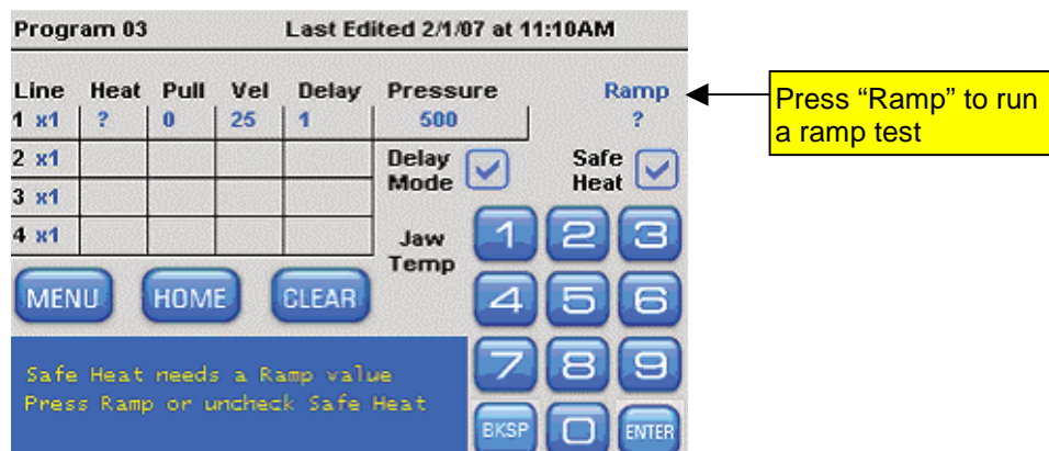
Figure 3-5. Running the ramp test.
