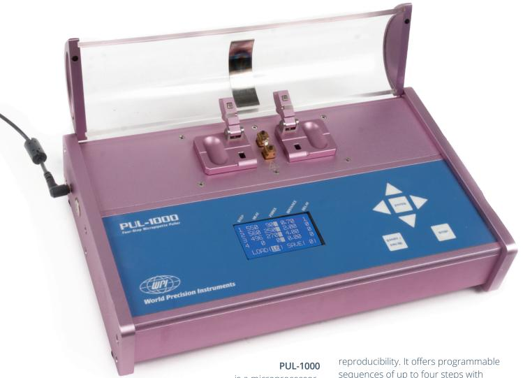
is a microprocessor controlled horizontal puller for making glass micropipettes or microelectrodes used in intracellular recording, microperfusion or microinjection. The puller was designed with tighter mechanical specifications and precision electronics for complete control of the pulling process and accurate
