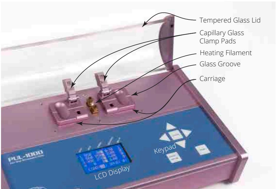
Fig. 2 The parts of the puller are identified.
