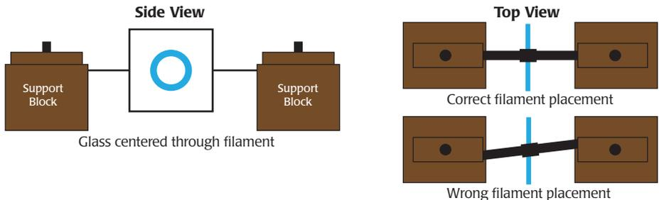
Fig. 12 Position the filament so the capillary glass runs through the center of the filament.
