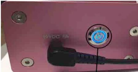
Fig. 5 The power is on, and the PUL-1000 switch is illuminated.
