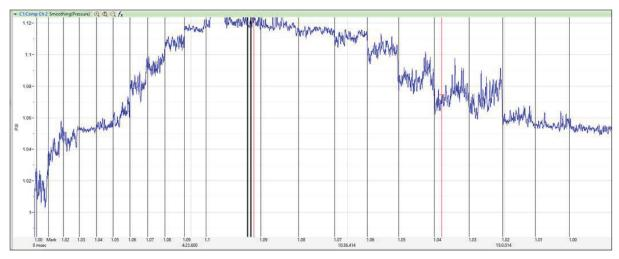
In the PV820, we attempted to perform the minimum movement necessary to induce a pressure change. The result was a minimum change of around .18 PSI (1.24106kpa). The settling time was between 18 and 22 seconds.
